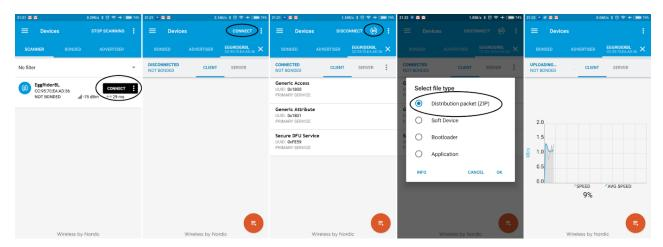
c) In case of firmware update the display will restart at the end of the process. In case of bootloader update, the display will shut down at the end of the process, and it will require a long power button press to start.
