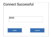
Enter the last 4 digits of the serial number as shown on the previous page (in this case it is 0055, but your BMS will be different). After entering the 4-digit number, press enter and you will be able to view the battery data.
