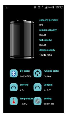
Now you are inside the app and can view various battery data, including total capacity, capacity remaining, instantaneous current and temperature. The capacity figures may require 1 or 2 cycles before the correct data is displayed.
