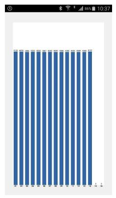
If you swipe right, you will be able to view the individual cell voltages for each cell in the battery. There are also additional pages for log data and the BMS configuration settings, which can be found by swiping right.
